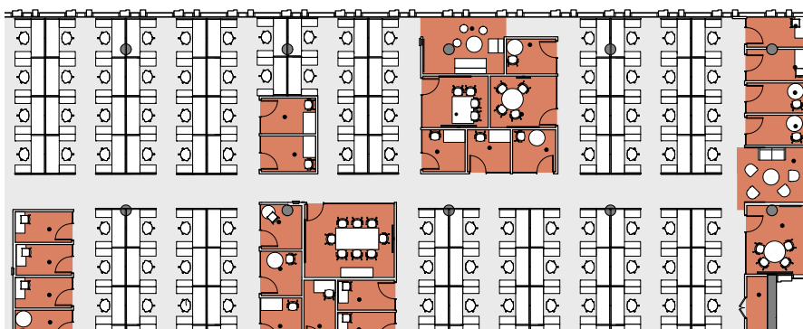
Below. In lieu of private offices, the Mission Hall floor plan features open offices with shared conference rooms.
